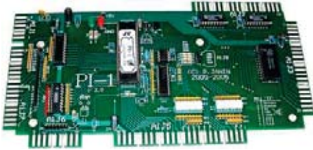
Pascal Janin's Pi-1 CPU replacement for Gottlieb System 1 machines
