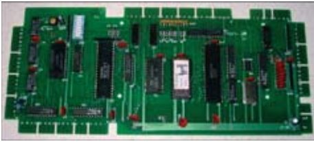
The Ni-Wumph Replacement CPU board for all Gottlieb System 1 machines.
