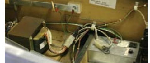
Above: Pinbot Filter cap and bridge rectifiers Below: ST:TNG transformer and service outlet
